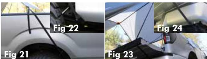
**14-**Run the tailgate straps around the tailgate and loosely attach to the lip of the bumper (Fig 23, Fig 24).
